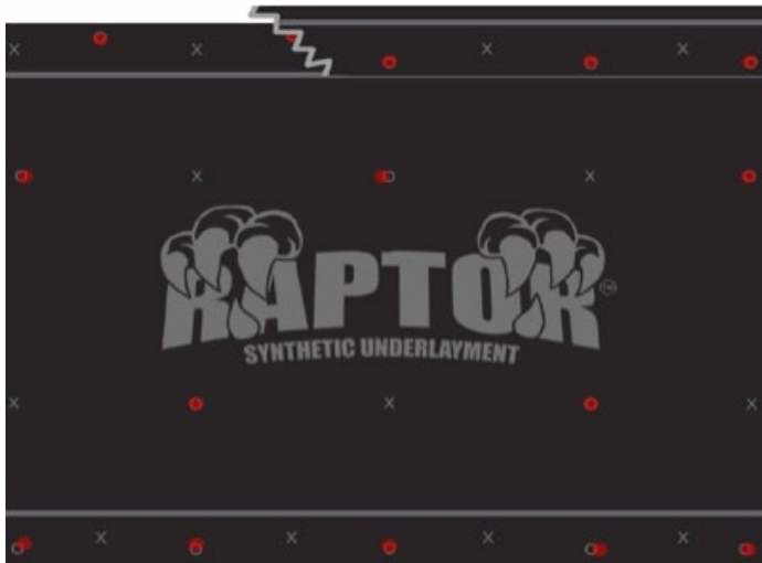
Nailing Pattern For Raptor In Normal Conditions Using Regular Roofing Nails or Cap Nails
